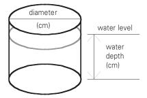
**FORMULA 1:** Volume (in litres) =  $0.8 \times \text{water depth (cm)} \times \text{diameter}^2 \text{ (cm}^2\text{)} \div 1000 \text{ (above diagram)}$
