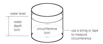
**FORMULA 2:** Volume (in litres) =  $0.08 \times \text{water depth (cm)} \times \text{circumference}^2 \text{ (cm}^2\text{)} \div 1000 \text{ (above diagram)}$
