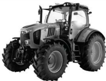
KUBOTA M7 152 STANDARD (DELUXE FITOUT) 6.1LTR KUBOTA ENGINE PRODUCING 148HP @ 1900RPM 30F/15R SPEED POWER SHIFT TRANSMISSION 50KM/H TRAVEL SPEED CABIN, AND FRONT AXLE SUSPENSION
